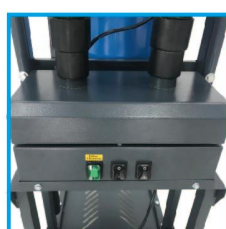
Individual switches control the 2 motors separately
