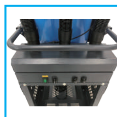
Individual switches control the 3 motors separately
