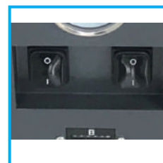
Individual switches control the 2 motors separately
