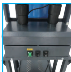
Individual switches control the 2 motors separately
